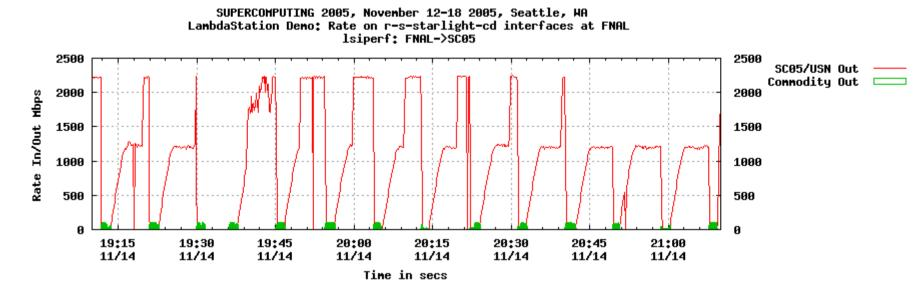
Tickets were placed periodically by application to switch its flows via 10G direct path from SC05/Seattle to Fermilab/Chicago.
