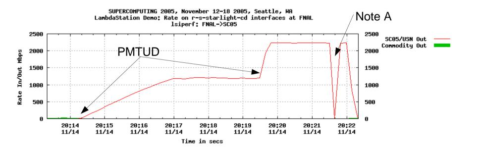
**Note A**: This dip has been identified as statistics gathering anomaly, believe to be an ASIC problem associated with router hardware. Measurement of the same throughput by other means (e.g. applications statistics) does not show that drop of rate..
