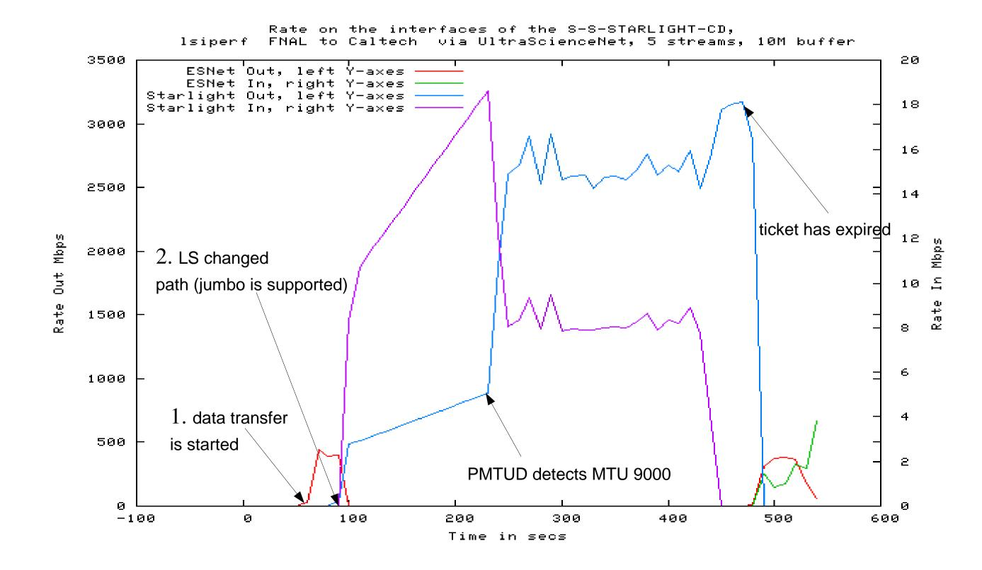
The graphs below show the results of performance measurements for flow based switching during Super Computing 2005, Seattle, WA, November 12 - 18, 2005. Two sites, Fermilab/Chicago and SC05/Seattle, were prepared to run this demo. At each site there were two test machines with 10G interfaces and one server running as a site LambdaStation (LS). Two alternative paths were available, the commodity Internet and the 10G path from the SC05 booth to the StarLight POP in Chicago and then to Fermilab.
